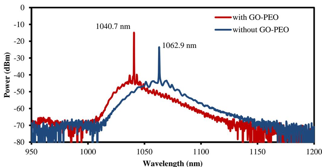
Fig. 4: The output OSA's spectra from the YDFL configuration with and without the GO-PEO SA at pump power of 111 mW
