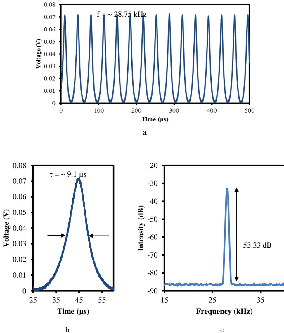
Fig. 6: (a) Oscilloscope trace for the YDFL with GO-PEO based SA at 111 mW pump power showing a repetition rate of 28.75 kHz; (b) Enlarged single envelop of the pulse (c) RF spectrum
