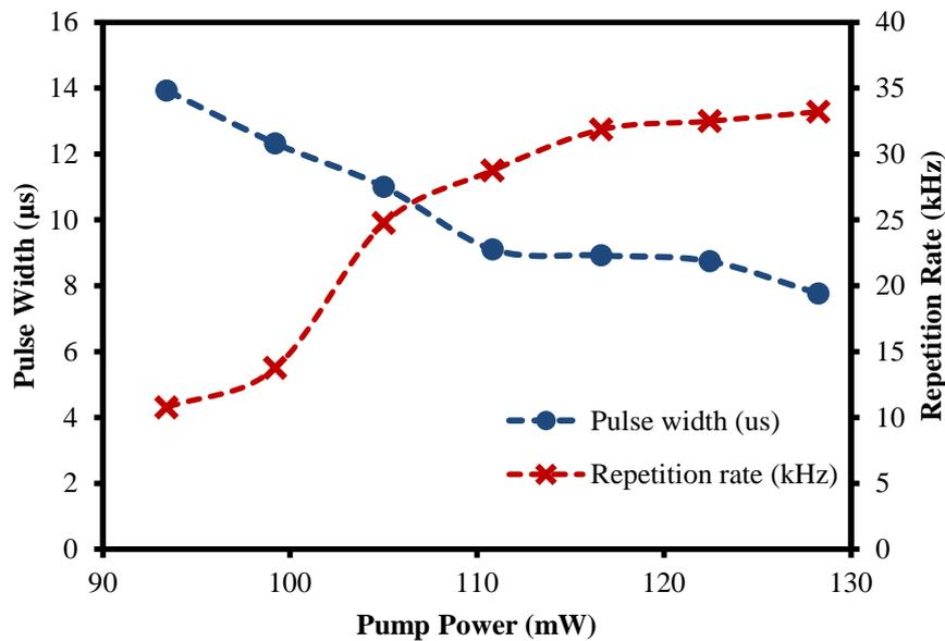
Fig. 5: Repetition rate and pulse width as a function of pump power.
