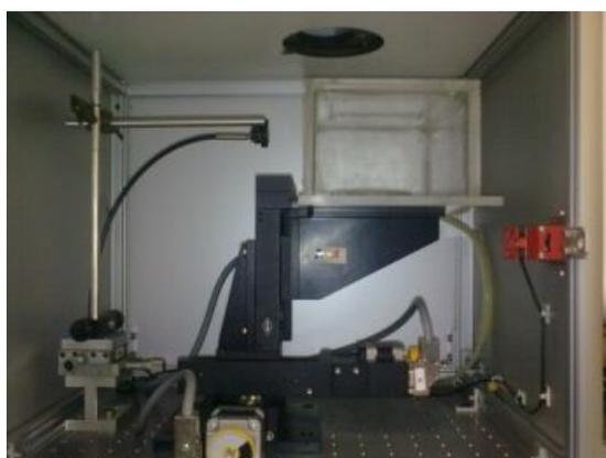
Fig. 1a. Experimental setup for laser induced breakdown spectroscopy (LIBS). b. Photograph of the sample analysis chamber.
