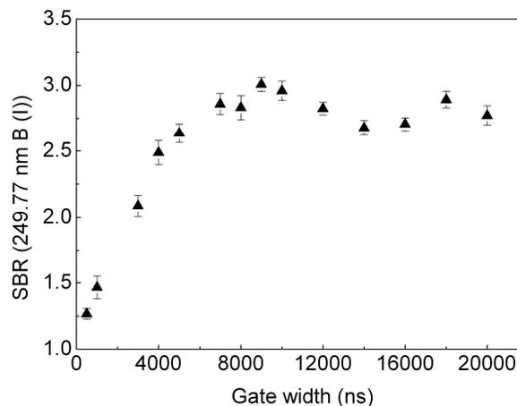
Fig. 5. Effect of the gate width on the SBR for the 249.7 nm boron emission line. Delay time = 1000 ns, slit width = 10  $\mu$ m, Gain = 230.
