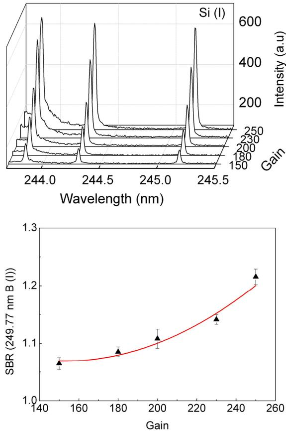
Fig. 6. Influence of intensifier gain. Delay time = 1000 ns, gate width = 7000 ns, slit width = 10  $\mu\text{m}$ .
