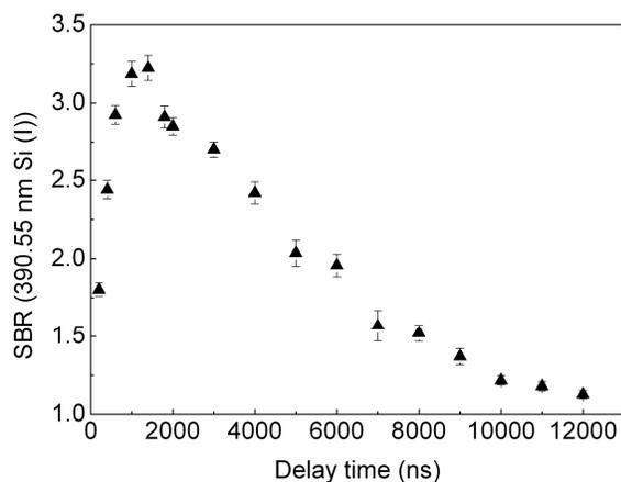
Fig. 3. Effect of the delay time on the SBR for the 390.5 nm silicon line. Gate width = 200 ns, slit width = 10  $\mu$ m, Gain = 230.
