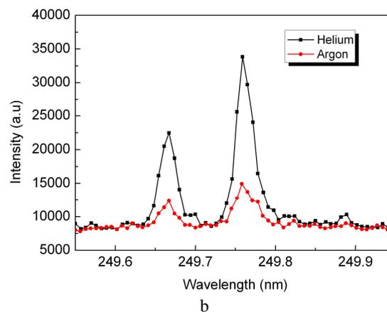
Fig. 2.a. Distribution of 100 single shots in helium atmosphere. b. Comparison between argon and helium atmosphere on the 249.6 and 249.7 nm boron line intensities with gating parameters having been determined separately for each gas. Delay time = 400 ns (He) and 1300 ns (Ar), gate width = 7000 ns (He) and 8000 ns (Ar), Gain = 190, slit width = 50  $\mu\text{m}$ , helium flow = 5.6 L.min<sup>-1</sup>.
