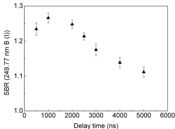
Fig. 4. Effect of delay time on the signal to background ratio for the 249.7 nm Boron line. Gate width = 500 ns, slit width = 15  $\mu$ m, Gain = 230.
