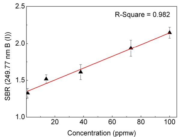
Fig. 7. Calibration curve for boron in certified standard silicon. Delay time = 1000 ns, gate width = 7000 ns, slit width = 50  $\mu\text{m}$ , Gain = 250.
