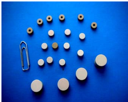
Fig. 2 X-ray diffraction pattern of ZST ceramic material. ZST cylindrical samples.
