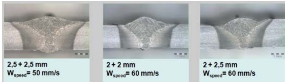
Fig. 9. LHW joints of DP 1000 steel sheets with filler material using LHW in keyhole mode at CLUPM.
