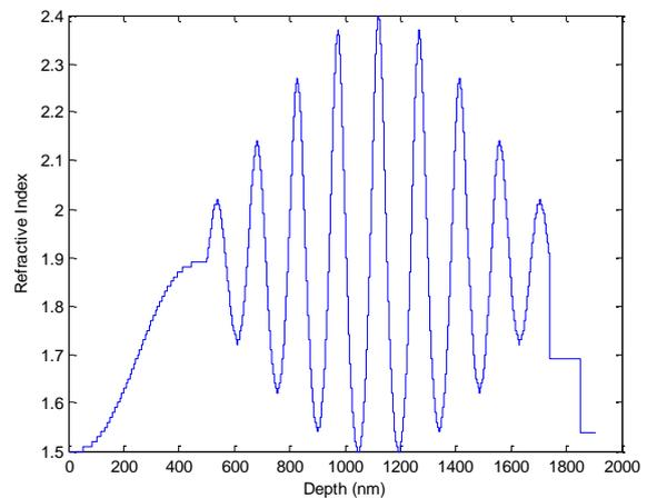
Fig. 10. Rugate filter with apodization, quintic matching layer, and top AR coating refractive index vs. depth (color online)
