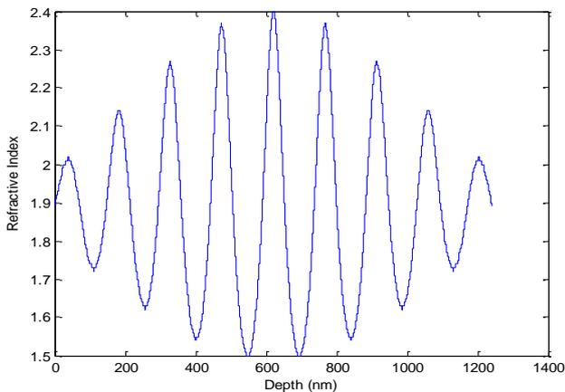
Fig. 4. Rugate filter with apodization refractive index on fused silica substrate vs. depth after applying apodization layers (color online)
