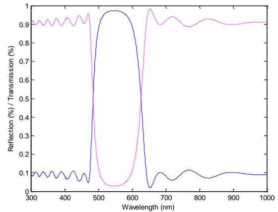
Fig. 9. Rugate filter with apodization and quintic matching layer reflection (continues line)/ transmission (dashed line) vs. wavelength (color online)
