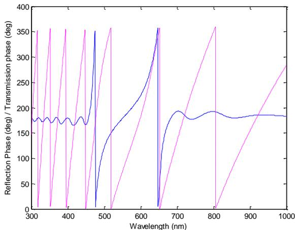
Fig. 8. Rugate filter with apodization and quintic matching layer reflection phase (continues line)/ transmission phase (dashed line) vs. wavelength (color online)
