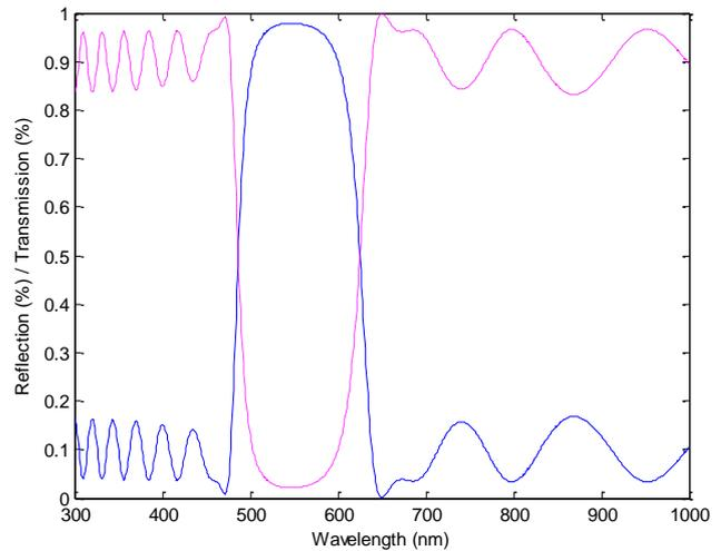
Fig. 6. Rugate filter with apodization reflection (continues line)/ transmission (dashed line) vs. wavelength (color online)
