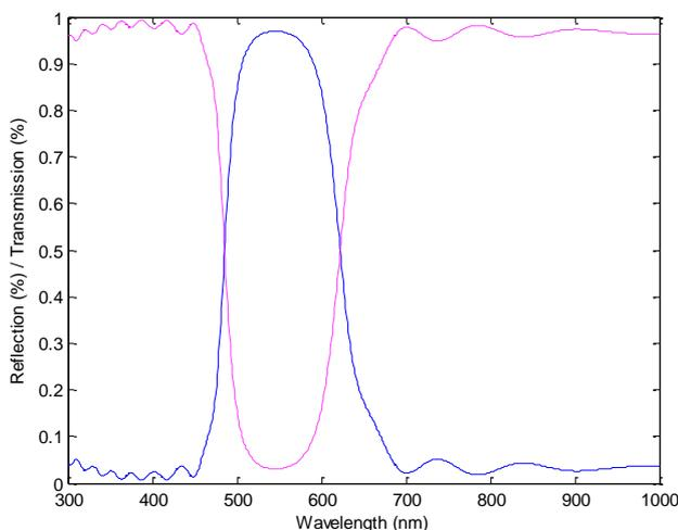
Fig. 12. Rugate filter with apodization, quintic matching layer, and top AR coating reflection (continues line)/ transmission (dashed line) vs. wavelength (color online)
