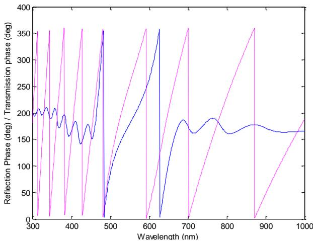
Fig. 11. Rugate filter with apodization, quintic matching layer, and top AR coating reflection phase (continues line)/ transmission phase (dashed line) vs. wavelength (color online)
