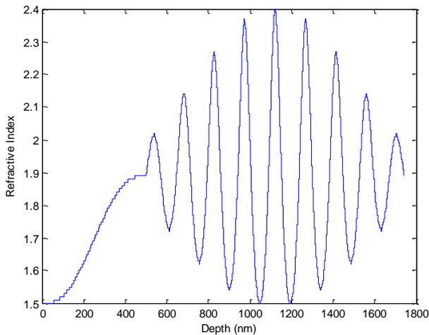
Fig. 7. Rugate filter with apodization and quintic matching layer refractive index vs. depth (color online)
