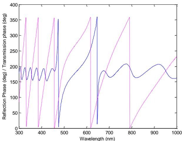
Fig. 5. Rugate filter with apodization reflection phase (continues line)/ transmission phase (dashed line) vs. wavelength (color online)
