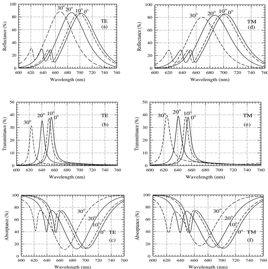
Fig. 2. The calculated reflectance, transmittance, and absorptance for TE wave ((a)-(c)) and TM wave ((d)-(f)) at various angles of incidence. Here the numbers of periods ( $m_1, m_2, m_3, m_4$ ) = (1, 3, 1, 3) are taken.
