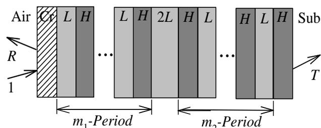
*Fig. 1. A narrow band reflection and transmission filter. The ultrathin metallic film, Cr, is deposited on FPR with a low-index defect layer, 2L. The reflectance and transmittance are R and T, respectively.*
