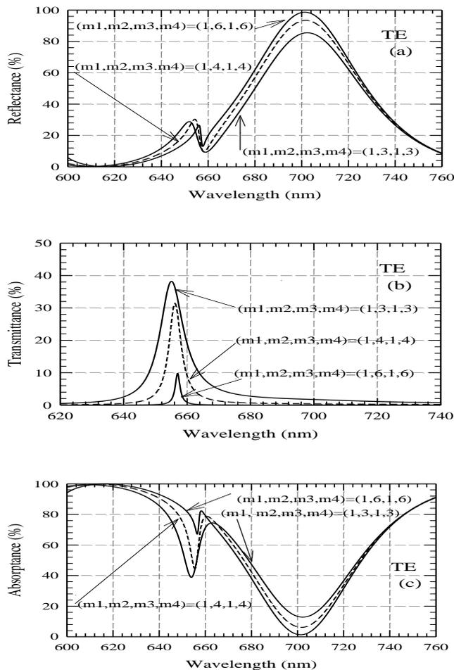
Fig. 5. The calculated  $R$ ,  $T$ , and  $A$  for the TE wave ((a)-(c)) at different combinations of  $(m_1, m_2, m_3, m_4)$ . Here the heterostructure is again with Fe in the second stage.
