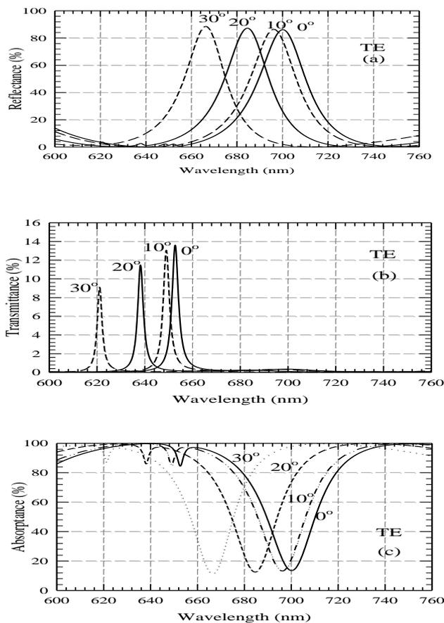
Fig. 3. The calculated  $R$ ,  $T$ , and  $A$  for the TE wave ((a)-(c)) at the numbers of periods  $(m_1, m_2, m_3, m_4) = (2, 4, 2, 4)$ .
