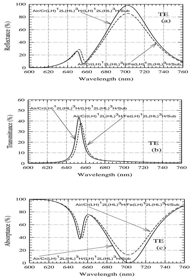
Fig. 4. The calculated  $R$ ,  $T$ , and  $A$  for the TE wave ((a)-(c)) at the numbers of periods  $(m_1, m_2, m_3, m_4) = (1, 3, 1, 3)$ . Here the dash curve is for the heterostructure with Fe in the second stage, while the solid one is for the same structure without Fe. The design wavelengths for the first and second stages are 700 and 650 nm, respectively.
