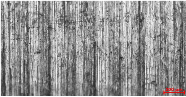
Fig.7 Lathed surface image of AlMgSi1 after 30 min
