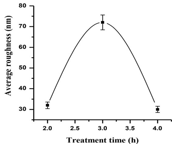
Fig. 5. The variation in surface roughness of P-ZnAlO films deposited for different ET.
