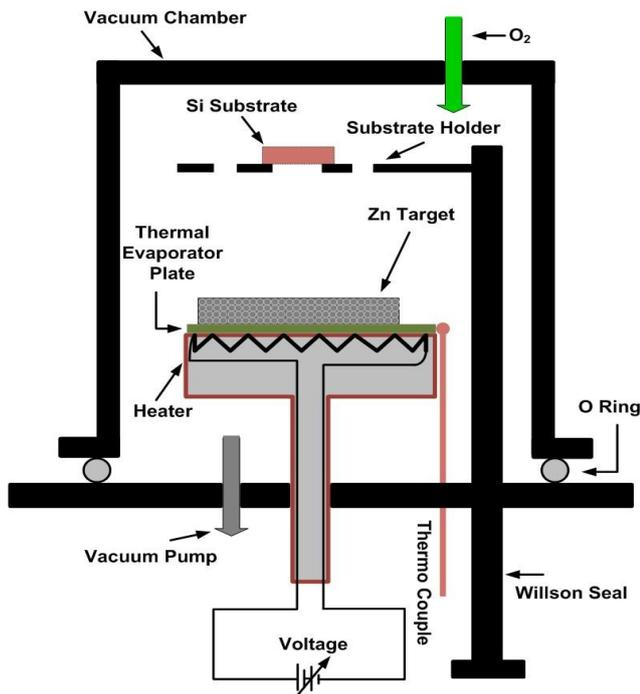
Fig. 1. The schematic diagram of thermal evaporator.
