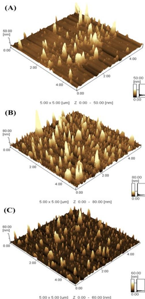
Fig. 4. The AFM images of the P-ZnAlO composite films deposited for (a) 2 hrs, (b) 3 hrs and 4 hrs ET.
