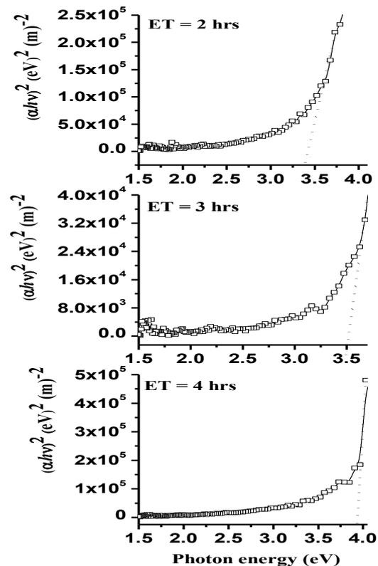
Fig. 7. The  $E_g$  of P-ZnAlO composite film deposited for 2, 3 and 4 hrs ET.
