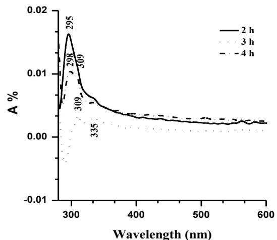
Fig. 6. The absorption spectra of P-ZnAlO composite films deposited for various ET.
