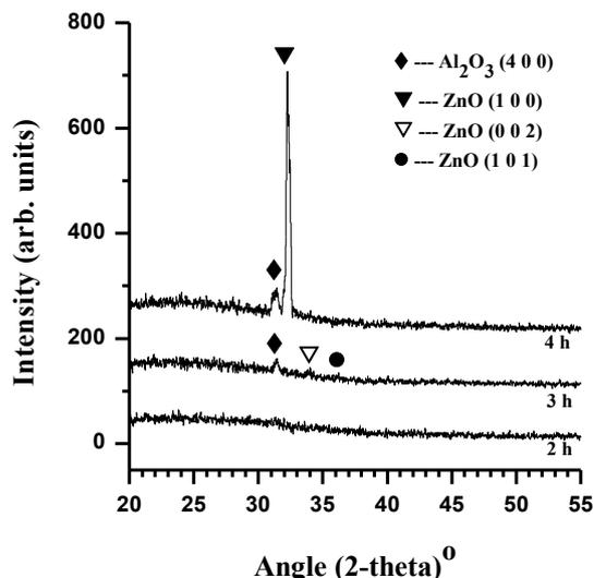
Fig. 2. The XRD patterns of P-ZnAlO composite films deposited for different ET.
