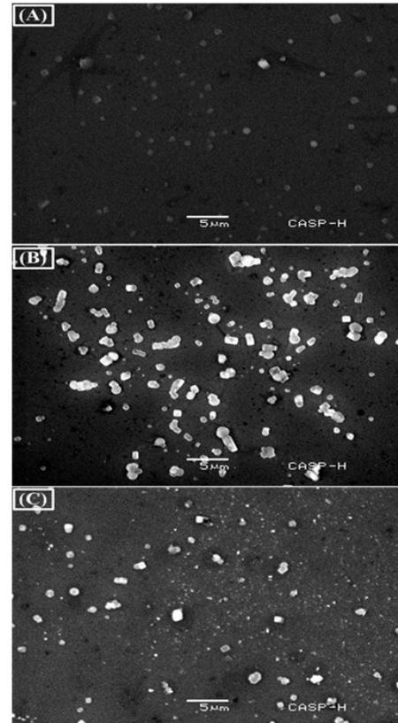
Fig. 3. The SEM microstructure of P-ZnAlO composite film deposited for (a) 2 hrs, (b) 3 hrs and (c) 4 hrs ET.
