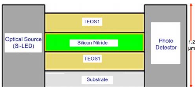
Fig. 6. Schematic presentations showing the basic design of the waveguides of the optical links, using silicon avalanche - based LED, silicon - based waveguide and Si-Ge based detectors.
