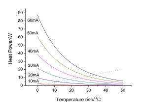
Fig. 6. Dependence of Joule heating power on glass wafer temperature rise (solid lines) in CC regime, with current value in the range from 10 to 60mA, at 10 mA intervals, and dependence of heat dissipation power on glass wafer temperature rise (dotted line)
