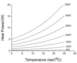
Fig. 2. Dependence of Joule heating power on glass wafer temperature rise (solid lines) in CV regime, and dependence of heat dissipation power on glass wafer temperature rise (dotted line).
