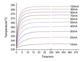
Fig. 5. Simulated glass wafer temperature rising in CC regime, with current value in the range from 10 to 100mA, at 10 mA intervals
