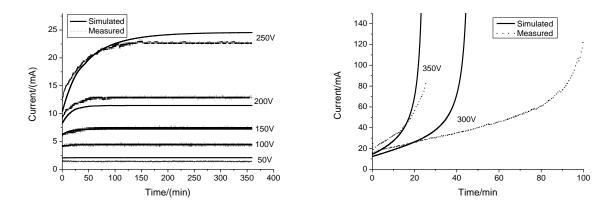
Fig. 3. Simulated and measured curves of current flowing through glass wafer in CV regime. Left: Voltage in the range from 50V to 250V at 50V intervals; right: voltage of 300V and 350V
