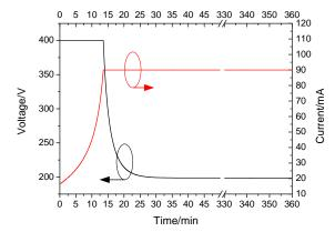
Fig. 9. Simulated voltage and current curves in the FAIM process in CV-CC regime
