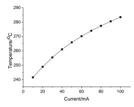
Fig. 7. Dependence of glass wafer temperature at equilibrium state on current in CC regime
