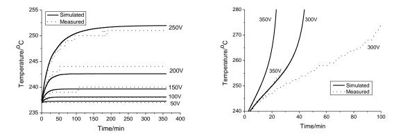
Fig. 1. Simulated and measured value of glass wafer temperature in CV regime. Left: Voltage in the range from 50V to 250V at 50V intervals; right: voltage of 300V and 350V
