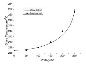
Fig. 4. Dependence of glass wafer temperature at equilibrium state on voltage in CV regime
