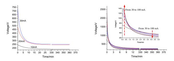
Fig. 8. Simulated value of voltage across glass wafer in CC regime. Left: current of 10mA, 20mA, and 30mA; right: current in the range from 30 to 100 mA, at 10 mA intervals. Insert in right image gives details of curves between in the beginning 5 minutes
