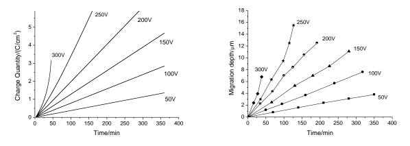
Fig. 10. Simulated charge quantity dependence on FAIM duration in CV regime (left), and measured value of migration depth dependence on FAIM duration in CV regime (right)
