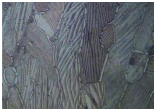
Fig. 2. Needle-shaped martensite and residual \beta phase in homogenized NMCG alloy at RT. x200
