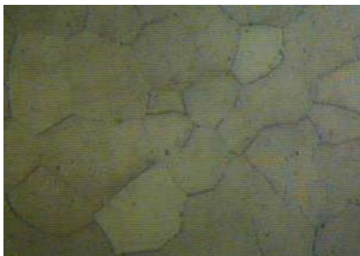
Fig. 1. The \beta solid solution structure of homogenized Ni 2 MnGa alloy at RT. x200.
