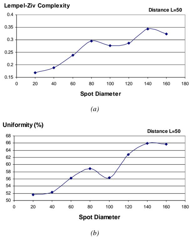
Fig. 5. LZC (a) and uniformity (b) vs. central spot diameter.
