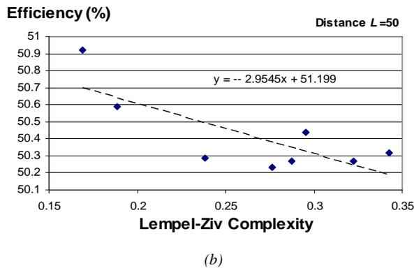
Fig. 7. Efficiency vs. central spot diameter (a), and anti-correlation between LZC and efficiency (b).
