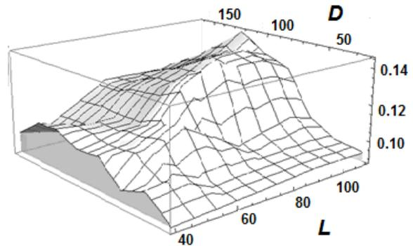
Fig. 2. MFS dependence on central spot diameter  $D$ , and inter-spot distance  $L$ .
