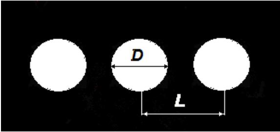
Fig.1. Signal window in triple beam configuration: central spot diameter  $D$ , and inter-spot distance  $L$ .
