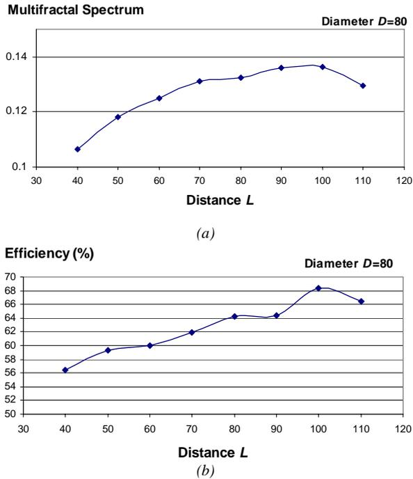
Fig. 3. MFS (a) and efficiency (b) vs. inter-spot distance.
