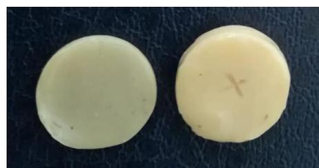
Fig. 2. The colour differentiation of the valid sample (left side) and the aged one (right side)
