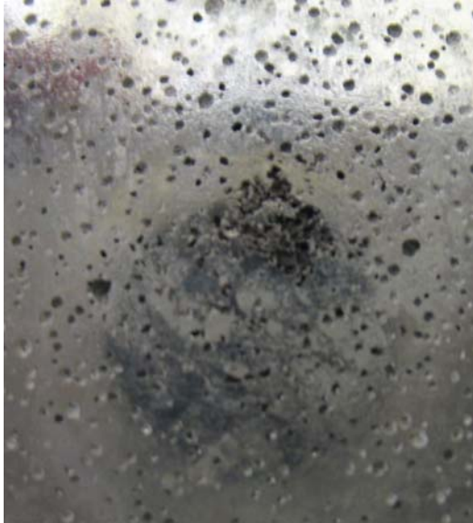
Fig. 5. Macroscopic image of AlMg15 metal foam.
