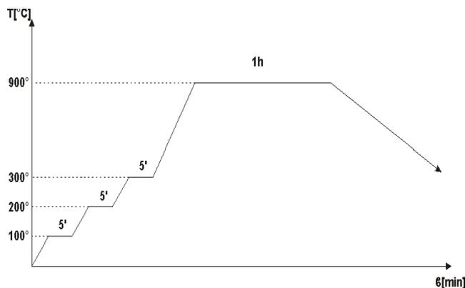
Fig.1. The graphical representation of the calcination process applied to HAP powders
