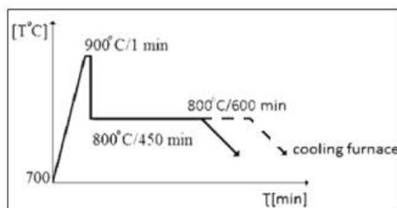
Fig.5. Graphical representation of the TSS process applied to HAP-based biocomposite
