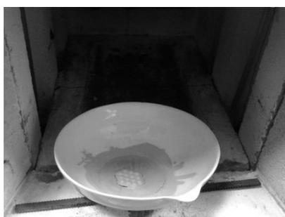
Fig.3. Drying of the biocomposite mixture HAP/Ti in the furnace after milling
