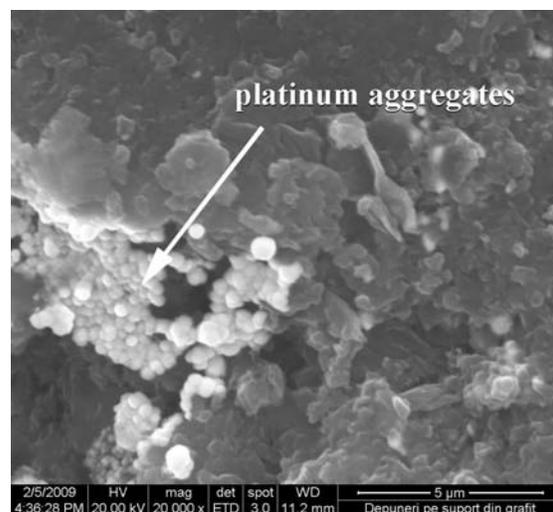
Fig. 7. SEM image of platinum electrodeposited catalyst in a micrometric porous sites of the carbon electrode with TiO<sub>2</sub> coating.
