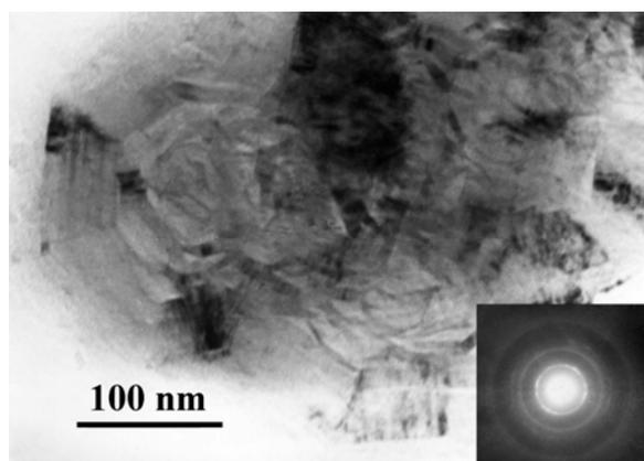
Fig. 1. TEM image and the corresponding SAED showing the nanostructure of the graphitized carbon supporting electrode.
