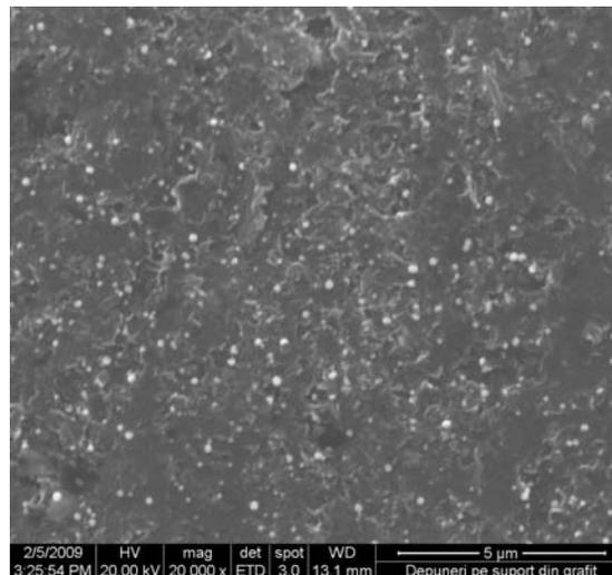
Fig. 2. The SEM image of carbon electrode decorated with small platinum particles
