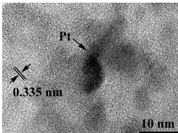
Fig. 4. High resolution TEM aspect of platinum nanoparticle embeded in the graphitized carbon matrix, which show the (0001) lattice fringes (0.335nm) characteristic for graphite.
