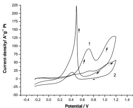
Fig. 11. Cyclic voltammograms for ethanol electro-oxidation at Pt/TiO<sub>2</sub>/G, (1) and Pt/G, (2) electrode in 3,75 M C<sub>2</sub>H<sub>5</sub>OH and 0.5 M H<sub>2</sub>SO<sub>4</sub> solution with a scan rate of 50 mV/s.
