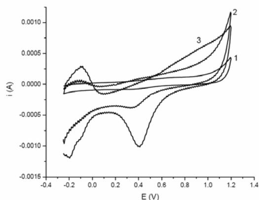
Fig. 10. CVs of the graphite (1),  $\text{Pt}/\text{G}$  (2) and the  $\text{Pt}/\text{TiO}_2/\text{G}$  electrodes (3).
