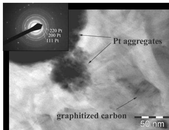
Fig. 3. TEM image and SAED pattern of platinum aggregate on carbon substrate.
