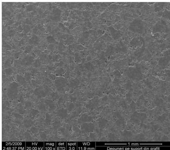
Fig. 5 Low magnification SEM image of the electrode covered surface with TiO<sub>2</sub> coating by electrochemical oxidation from TiCl<sub>3</sub> based solution at 0,7V/AgCl
