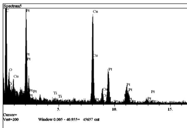
Fig. 8. EDX Spectrum of  $\text{TiO}_2/\text{Pt}$  hybrid system on the platinum covered sites.
