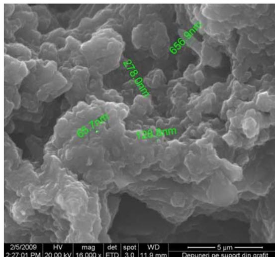
Fig. 6. SEM image of the three- dimensional grow of titanium dioxide coating.
