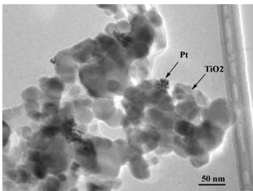
Fig. 9. High magnification TEM image showing platinum particle aggregate on the  $\text{TiO}_2$  particles.
