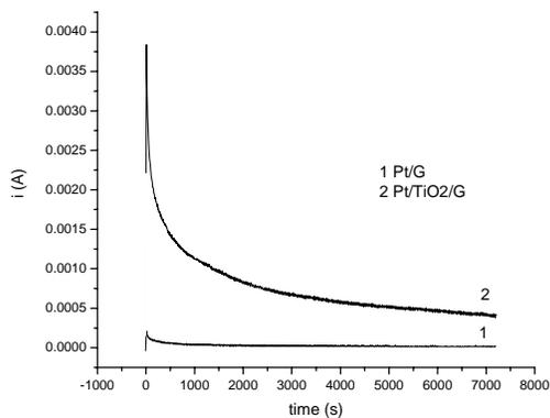
Fig. 12. Chronoamperometric response of Pt/G (1) and TiO<sub>2</sub>/Pt/G (2) electrodes of the ethanol oxidation in 0.5 M H<sub>2</sub>SO<sub>4</sub> solution at an applied potential of 0.6 V vs. Ag/AgCl.
