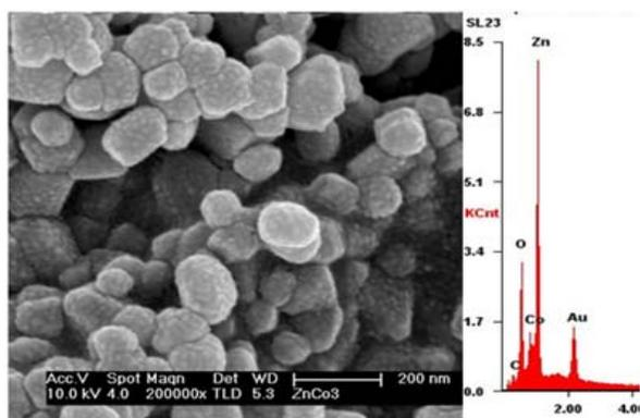
Fig. 4 SEM image of 5% Co doped ZnO powder along with EDAX pattern
