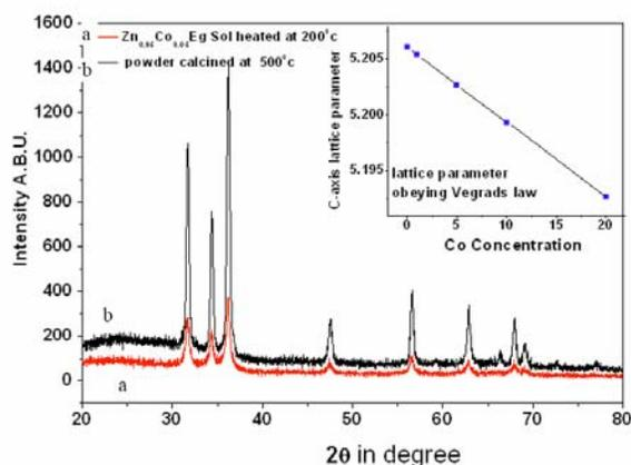
Fig. 2 XRD pattern of  $Zn_{0.95}Co_{0.05}O$  obtained by heating at different temperature
