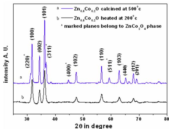
Fig. 3 XRD pattern of  $Zn_{0.8}Co_{0.2}O$  heated at  $200^\circ C$  and calcined at  $500^\circ C$
