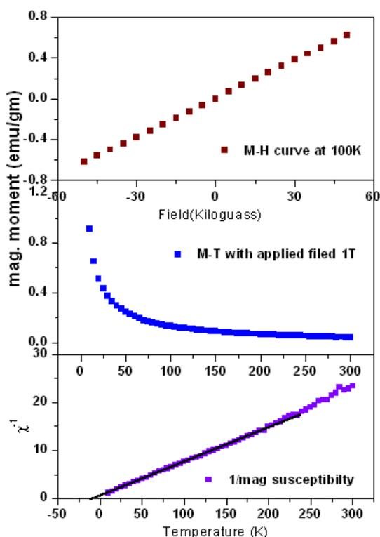
Fig. 5 magnetic moment of  $Zn_{0.9}Co_{0.1}O$  obtained by heating at different temperature.
