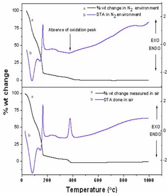
Fig. 1 DTA-TGA of  $Zn_{0.95}Co_{0.05}Eg$  complex in air and  $N_2$  environment.
