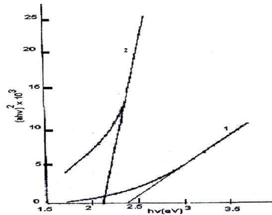
Fig. 4. Tauc's plot of: 1. Cd(S<sub>0.95</sub>-Se<sub>0.05</sub>) film, 2. Cd(S<sub>0.95</sub>-Se<sub>0.05</sub>):CdCl<sub>2</sub>,Pr film.
