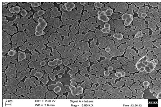
Fig.-1 SEM micrograph of chemically deposited Cd( $\text{Se}_{0.95}\text{-S}_{0.05}$ ):CdCl<sub>2</sub>,Pr film
