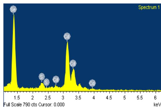
Fig.-2 EDX spectrum of chemically deposited Cd( $\text{Se}_{0.95}\text{-S}_{0.05}$ ) film.
