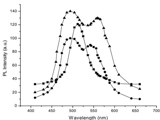
Fig.5. PL emission spectra of different  $Cd(S_{1-x}Se_x)$  films prepared at  $60^\circ C$  with different values of  $x$ : ■ CdS, ◆  $Cd(Se_{0.95}S_{0.05})$  and ▲  $Cd(Se_{0.95}S_{0.05}):CdCl_2$
