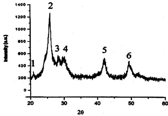
Fig. 3 X-ray diffractogram of Cd(Se<sub>0.95</sub>-S<sub>0.05</sub>):CdCl<sub>2</sub>,Pr film.
