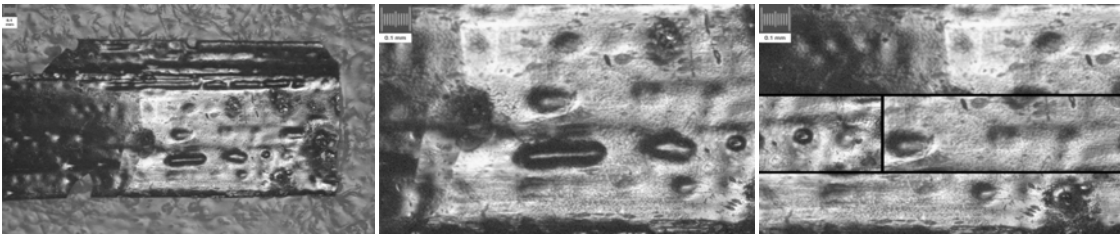
Fig. 8. The microscopically analyses for \text{Cu}_{50}\text{Zr}_{45}\text{Gd}_5 (glossy side of the ribbon)
