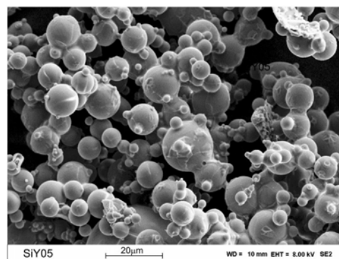
Fig. 1. BEI-SEM micrograph of SiY05 microspheres.
