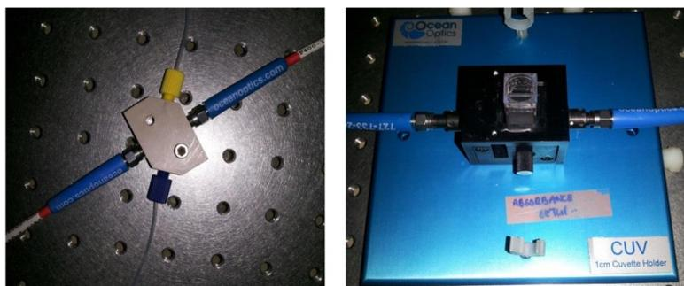
Fig. 2. Experimental setup: (a) Z-flow injection (b) Cuvette.
