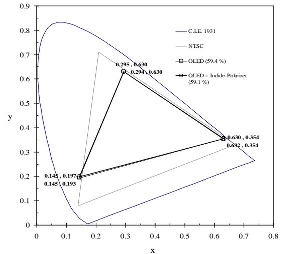
Fig. 6. The  $\text{CIE}_{1931}$  Chromaticity Diagram displays the  $\text{CIE}_{1931}$  index and color saturation of the OLED with and w/o an Iodide-Polarizer in the darkroom.
