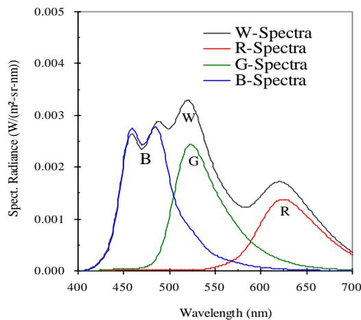
Fig. 2. The Spectra in the experimental PMOLED is turned on by driver IC @ 13.5V and measured by a Minolta Chroma Meter CS-1000 in a darkroom.
