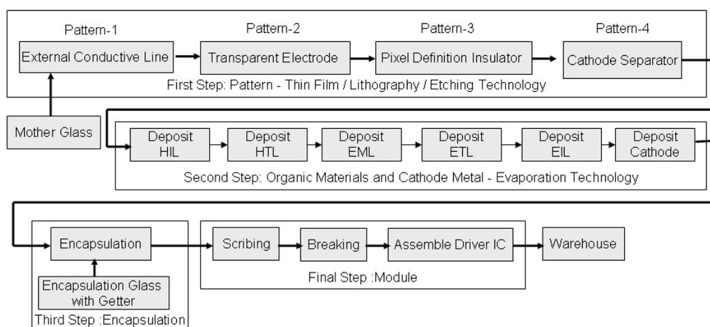
Fig. 1. The Process flow of panel in the PMOLED
