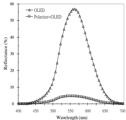
Fig. 4. The reflectance of the OLED with and w/o an iodide-polarizer for visual reflective sensitivity of human eyes.
