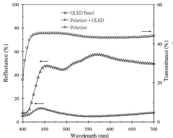
Fig. 3. Transmittance of an iodide-polarizer, reflectance of the OLED and applying an iodide-polarizer on the panel of the OLED. The transmittance and the reflectance are measured by Hitachi U4100 system.
