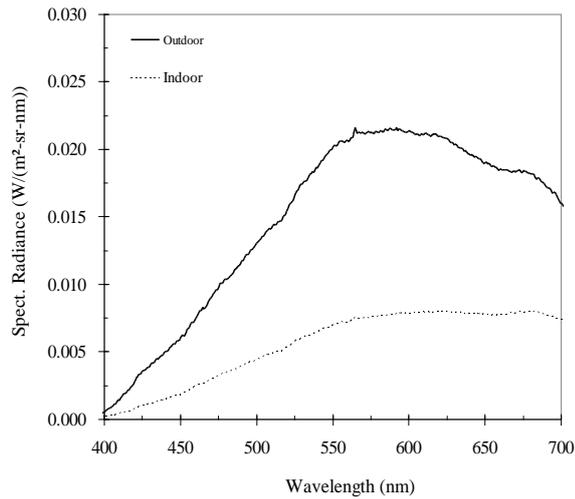
Fig. 5. The spectra of indoor ambience and outdoor ambience are simulated by the DMS-505 system of the autronic MELCHERS GmbH.
