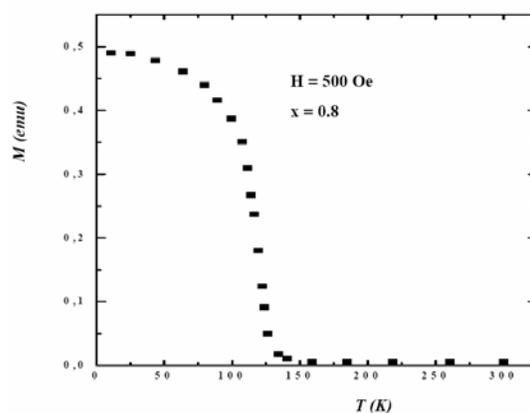
Fig 1. Temperature dependence of the magnetization at low field ( $H = 500\text{Oe}$ ) for the  $\text{CdGa}_{2-2x}\text{Cr}_{2x}\text{Se}_4$  ( $x = 0.8$ ).
