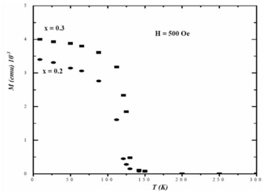
Fig. 3. Temperature dependence of the magnetization at low field ( $H = 500Oe$ ) for the  $CdGa_{2-2x}Cr_{2x}Se_4$  ( $x = 0.3, 0.2$ ).
