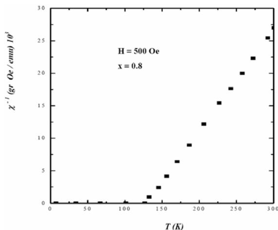
Fig 2. Temperature dependence of the inverse of the magnetic susceptibility at low field ( $H = 500\text{Oe}$ ) for the  $\text{CdGa}_{2-2x}\text{Cr}_{2x}\text{Se}_4$  ( $x = 0.8$ ).
