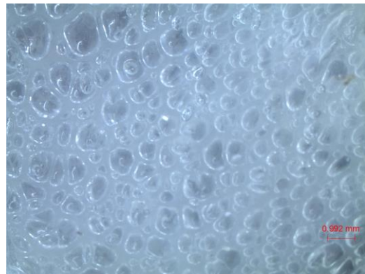
Fig. 6. The microstructure of PMI foam material (the mass ratio was 1:2).
