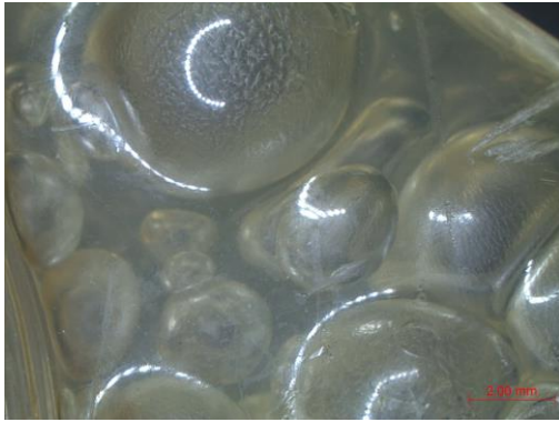
Fig. 3. The microstructure of PMI foam material (hexyl alcohol as the foaming agent).
