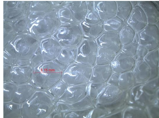
Fig. 5. The microstructure of PMI foam material (the mass ratio was 1:3).
