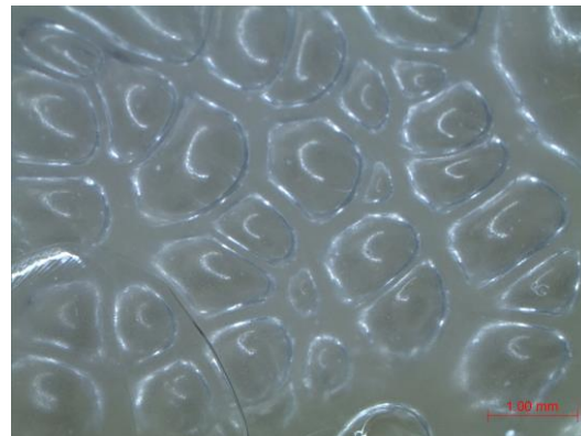
Fig. 7. The microstructure of PMI foam material (the mass ratio was 1:1).
