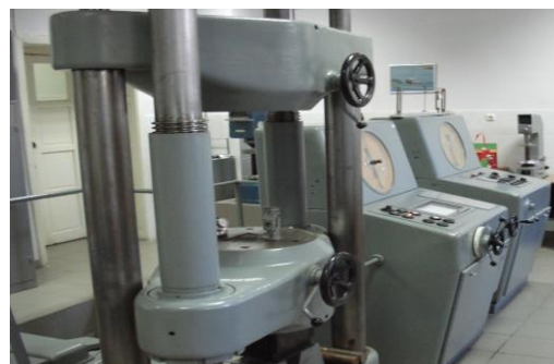
Fig.11. Universal Testing Machine used for testing tensile strength, compressive strength and bending strength of different materials.
