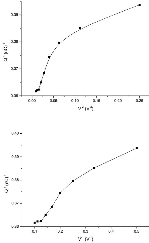
Fig. 2. Plot of a)  $1/Q$  vs.  $1/V^2$  and b)  $1/Q$  vs.  $1/V$  (so-called Jaffe plot) at constant dose.
