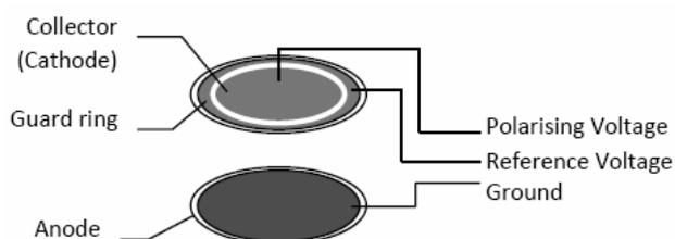
Fig. 1. Schematic of the designed charge collecting electrodes and its connections.
