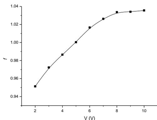
Fig. 3. Ion collection efficiency,  $f$ , of chambers vs. applied voltage for  $^{60}\text{Co}$  radiation.
