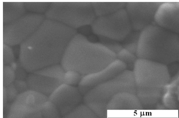
Fig. 12. SEM image of BMT sample with 0.25 mol %  $\text{Nb}_2\text{O}_5$ , sintered at 1650 C / 4h.
