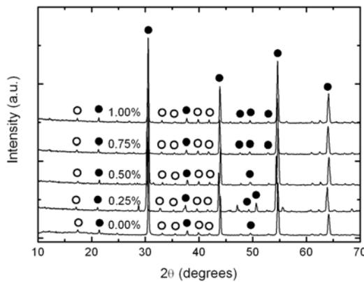
Fig. 5. XRD patterns of  $V^{5+}$  doped BMT ceramics for  $T_s = 1650$  °C: ● - BMT cubic structure reflections, ○ - BMT superstructure reflections.
