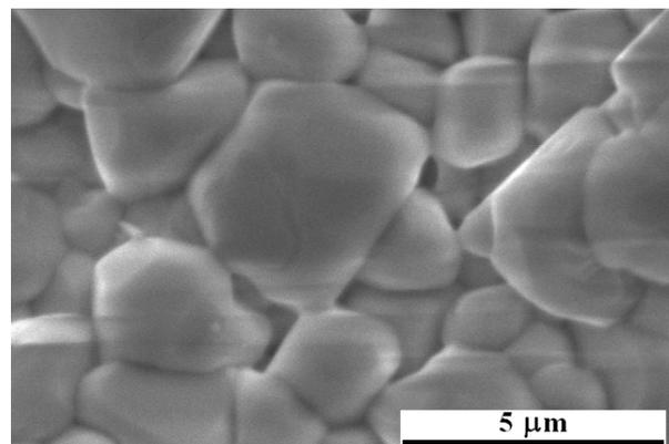
Fig. 13. SEM image of BMT sample with 0.50 mol %  $\text{V}_2\text{O}_5$ , sintered at 1600 C / 4h.
