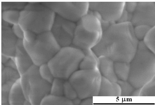
Fig. 10. SEM image of BMT sample with 0.50 mol %  $\text{Nb}_2\text{O}_5$ , sintered at 1600 C / 4h.
