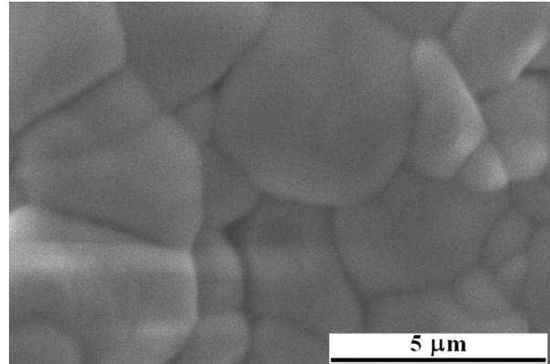
Fig. 11. SEM image of BMT sample with 0.50 mol %  $\text{Nb}_2\text{O}_5$ , sintered at 1650 C / 4h.
