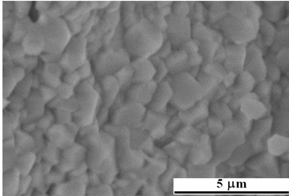
Fig. 8. SEM image of undoped BMT sample sintered at 1650 C / 4h.
