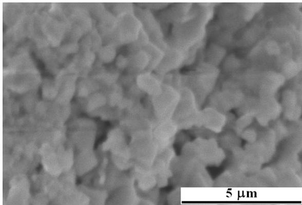
Fig. 9. SEM image of BMT sample with 0.50 mol %  $\text{Nb}_2\text{O}_5$ , sintered at 1550 C / 4h.
