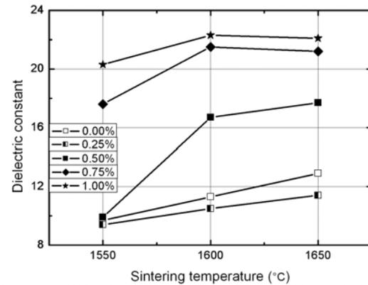
Fig. 16. Dielectric constant of BMT ceramics versus sintering temperature in the case of using  $Nb^{5+}$  as dopant.
