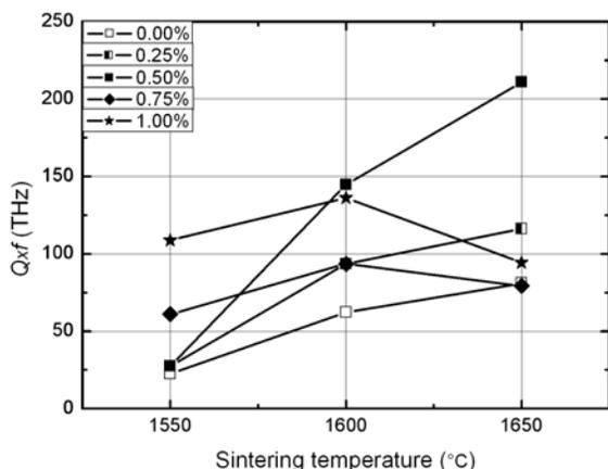
Fig. 18.  $Q \times f$  product of BMT ceramics versus sintering temperature in the case of using  $\text{Nb}^{5+}$  as dopant.
