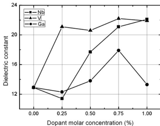
Fig. 15. Dielectric constant of BMT ceramics versus molar concentration of dopant ( $Nb_2O_5$ ,  $V_2O_5$ ,  $Ga_2O_3$ ) for  $T_s = 1650\text{ }^\circ\text{C}$ .
