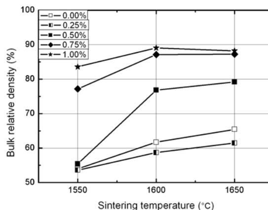
Fig. 3. Bulk relative density of BMT ceramics versus sintering temperature in the case of using Nb<sup>5+</sup> as dopant.
