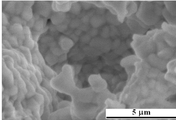
Fig. 14. SEM image of BMT sample with 0.25 mol %  $Ga_2O_5$ , sintered at 1650 C / 4h.
