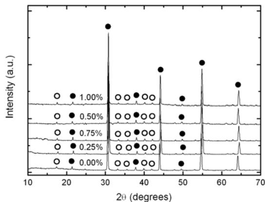
Fig. 6. XRD patterns of  $Ga^{3+}$  doped BMT ceramics for  $T_s = 1650$  °C: ● - BMT cubic structure reflections, ○ - BMT superstructure reflections.
