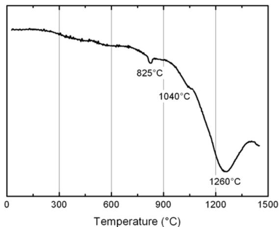
Fig. 1. DSC analysis of the precursor powders mixture.
