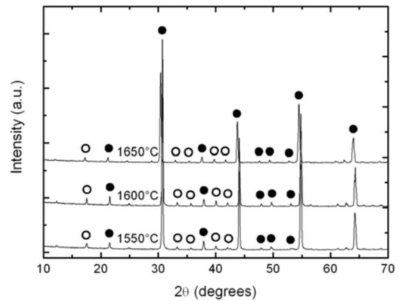
Fig. 7. XRD patterns of BMT ceramics with 0.50 mol %  $Nb_2O_5$ : ● - BMT cubic structure reflections, ○ - BMT superstructure reflections.
