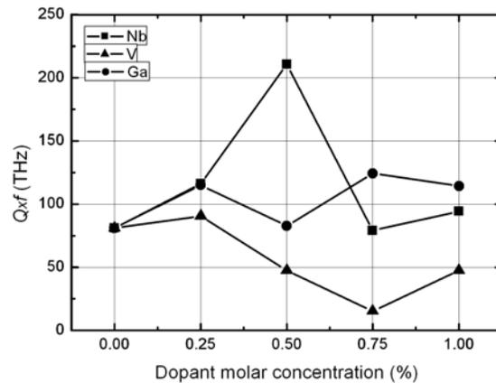
Fig. 17.  $Q \times f$  product of BMT ceramics versus molar concentration of dopant ( $Nb_2O_5$ ,  $V_2O_5$ ,  $Ga_2O_3$ ) for  $T_s = 1650\text{ }^\circ\text{C}$ .
