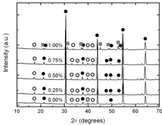
Fig. 4. XRD patterns of  $Nb^{5+}$  doped BMT ceramics for  $T_s = 1650$  °C: ● - BMT cubic structure reflections, ○ - BMT superstructure reflections, ■ - unknown phase.
