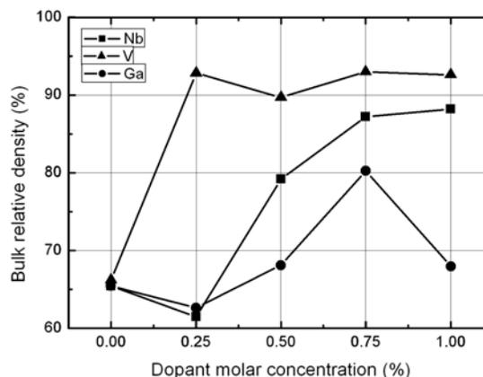
Fig. 2. Bulk relative density of BMT ceramics versus molar concentration of dopant (Nb<sub>2</sub>O<sub>5</sub>, V<sub>2</sub>O<sub>5</sub>, Ga<sub>2</sub>O<sub>3</sub>) for  $T_s = 1650$  °C.
