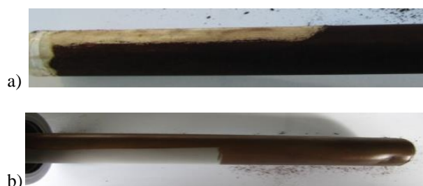
Fig. 3. Nanopowders are collected simultaneously on a ceramic filter (a) and on water cooled copper finger (b)
