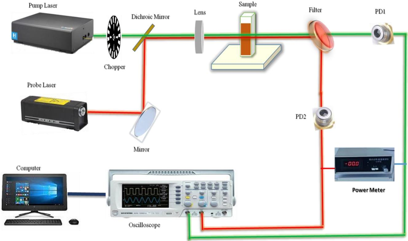
Fig. 5. The pump-probe experimental setup for optical switching measurements (color online)
