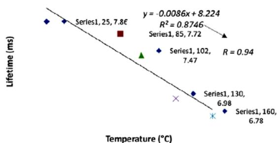
Fig. 4. Lifetime of EDF as function of Temperature.
