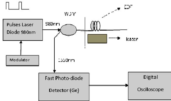
Fig. 1. Experiment setup of fiber optic high temperature sensor.
