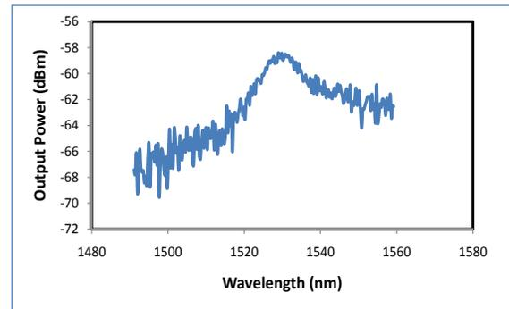
Fig. 2. Output spectrum of the generated ASE with 980 nm pump power of 31mW.
