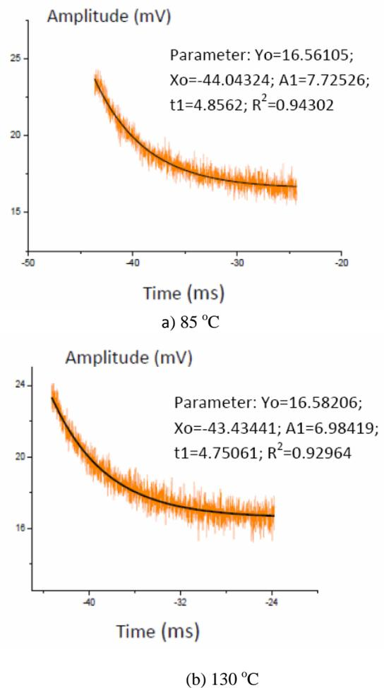
Fig. 3. Fluorescence lifetime decay of EDF at (a) 85 °C and (b) 130 °C from a digital oscilloscope.
