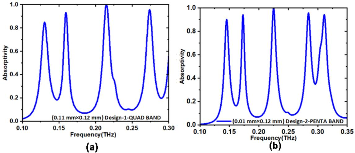
Fig. 4. Quad band and Penta band operation of an MMA (color online)
