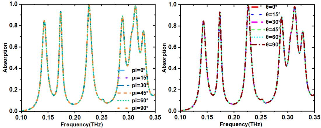
Fig. 8. Polarization ( $\phi$ ) and angle insensitivity ( $\theta$ ) of the MMA (color online)
