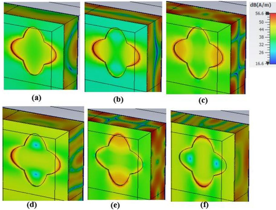
Fig. 10. Magnetic field distribution of MMA for six bands (a) 0.146 THz, (b) 0.174 THz, (c) 0.227 THz, (d) 0.288 THz, (e) 0.315 THz, (f) 0.328 THz (color online)
