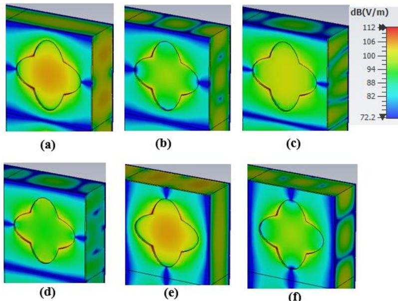
Fig. 9. Electric field distribution of MMA for six bands (a) 0.146 THz, (b) 0.174 THz, (c) 0.227 THz, (d) 0.288 THz, (e) 0.315 THz, (f) 0.328 THz (color online)
