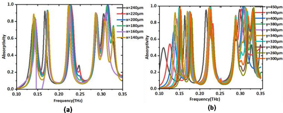
Fig. 7. Parametric study for hexa band operation in etched eclipse shaped patch structure (color online)
