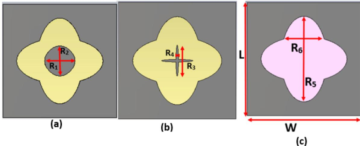
Fig. 2. Different developing stages of the quad-/penta and hexa band MMA (a) Quad band (b) Penta band (c) Hexa band, (Grey colour represents the copper, yellow and pink layer represents the polyimide substrate) (color online)
