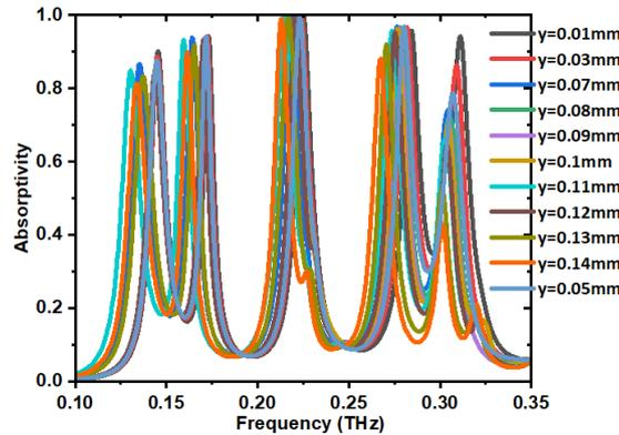
Fig. 6. Parametric study for quad and penta band operation in inner eclipse shaped patch structure (color online)
