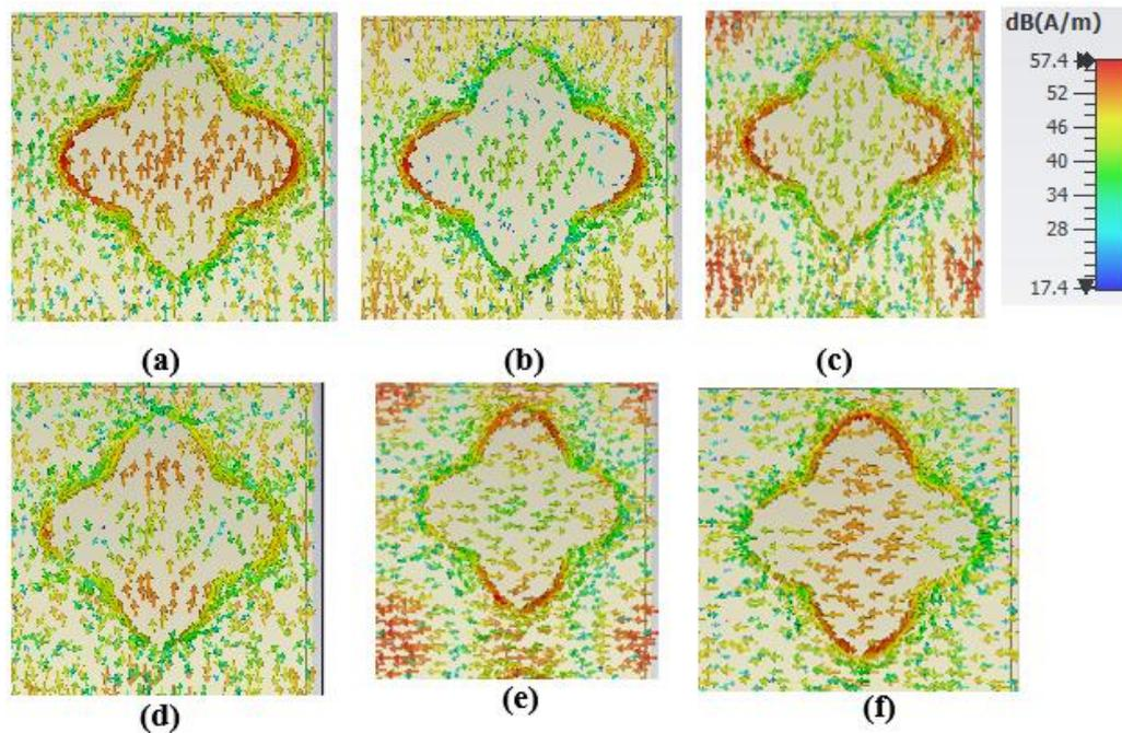
Fig. 10. Surface current distribution of MMA for six bands (a) 0.146 THz, (b) 0.174 THz, (c) 0.227 THz, (d) 0.288 THz, (e) 0.315 THz, (f) 0.328 THz (color online)
