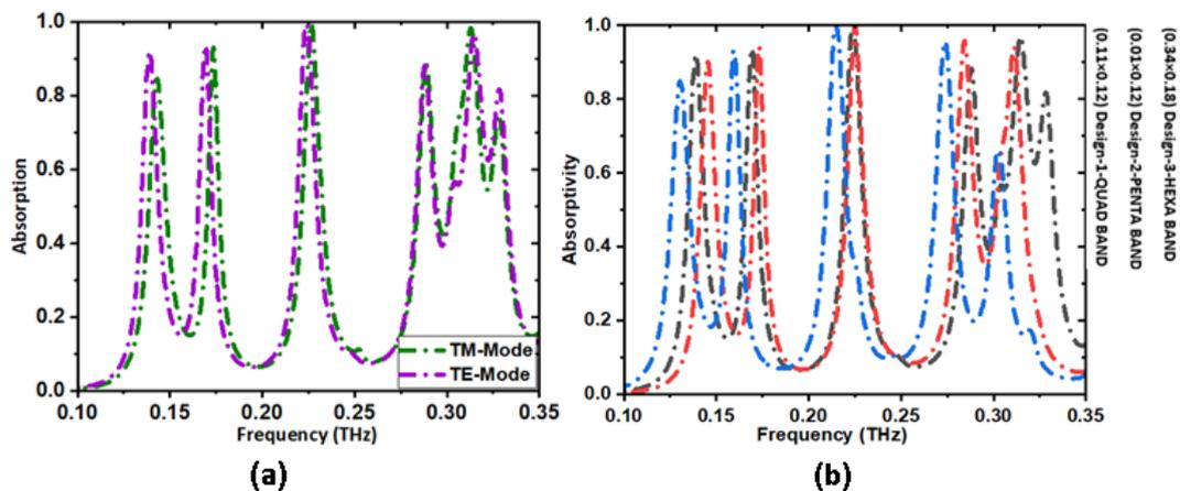
Fig. 5 (a). Hexa band operation of an MMA, (b) Comparison graph for quad-/penta and hexa band operation (color online)
