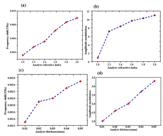
Fig. 3. (a) Frequency shift versus analyte refractive index, (b) Amplitude modulation versus analyte refractive index at a top layer thickness of 50µm, (c) (d) Frequency shift and amplitude modulation versus analyte thickness (color online)
