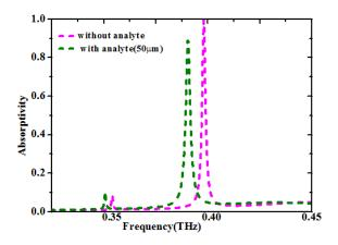
Fig.2. (a) Simulated absorption curves with a 50-µm-thick analyte and without analyte (color online)
