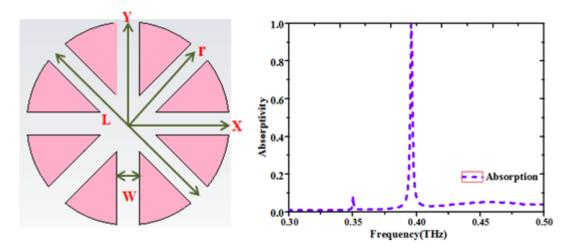
Fig.1. (a). Geometrical parameters of the metamaterial unit cell (r=0.16mm, l=0.32mm, w=0.036mm), 1(b) Absorption curve for the proposed absorber (color online)
