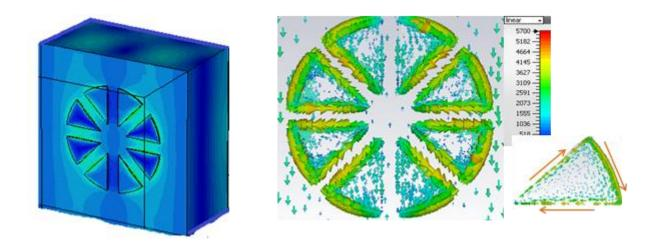
Fig.4. (a).Distributions of the magnetic field for the proposed terahertz sensor at a frequency of 0.3956 THz, (b) Surface current distribution and direction of the current flow (color online)
