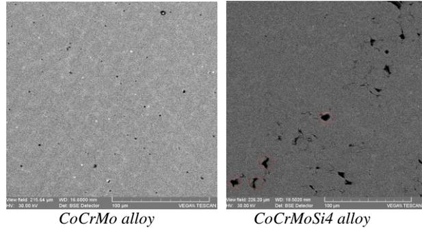
Fig. 7. Microstructure of investigated alloy - 1000X BSE magnitude.
