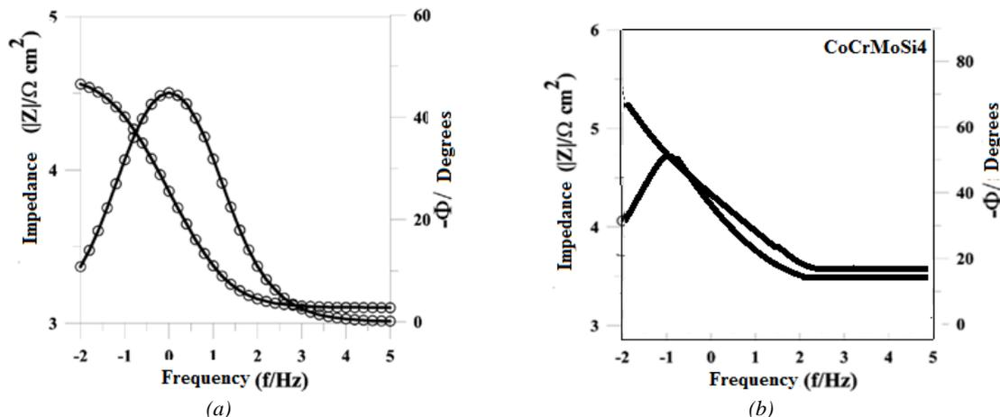
Fig. 3. Bode diagrams for studied alloys: (a) commercial alloy from CoCrMo system and (b) CoCrMoSi4 experimental alloys, maintaining for 750 seconds in fresh orange juice, unpasteurized.
