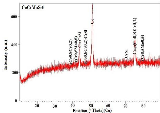
Fig. 2. X-ray diffractogram (indexed) obtained for CoCrMoSi4 alloy.
