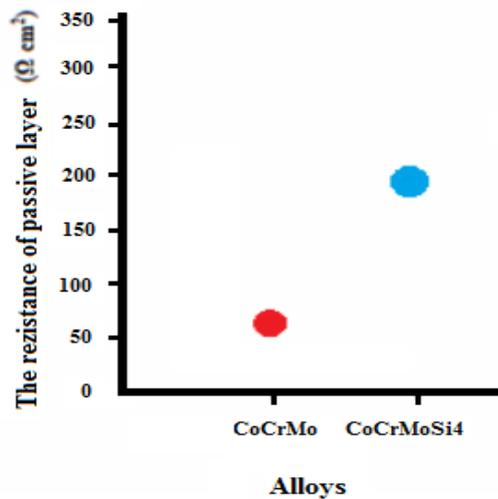
Fig. 5. Graphic representation for passive layers resistance, for new alloy, maintaining for 750 seconds in fresh orange juice, unpasteurized.
