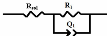
Fig. 4. Equivalent circuit (CE) used in experimental data filtering, obtained for CoCrMo commercial alloys, maintained in fresh orange juice, unpasteurized. [14].
