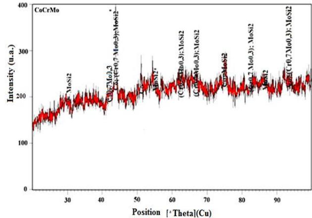
Fig. 1. X-ray diffractogram de raze X (indexed) obtained for CoCrMo commercial alloy.
