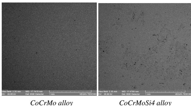
Fig. 6. Microstructure of investigated alloy – 100X BSE magnitude.
