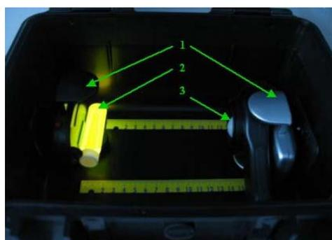
Fig. 2 B&W case: 1. Fixing systems, 2. 10 ml vials with CL composition, 3. Extech HD 450 sensor.
