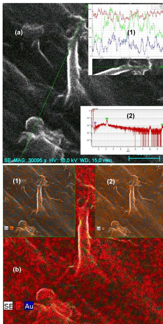
Fig. 3. Linear profile surface microanalysis (a) and corresponding chemical mapping (b) in the case of a LDPE sample
