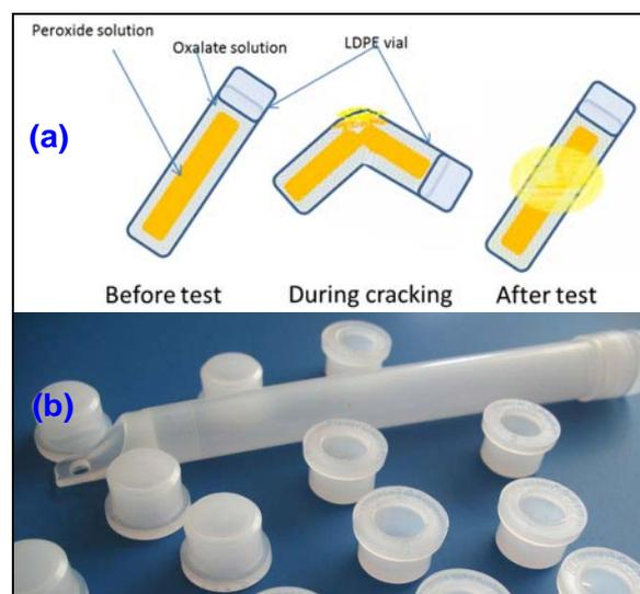
Fig. 6. The working principle of the light stick (a) and the final product (b)
