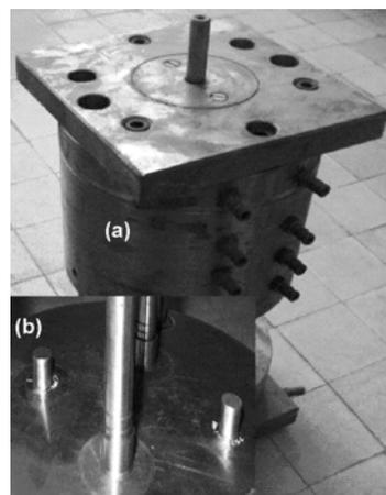
Fig. 1. The plastic vials and plastic caps injection molding equipment (a) and its particular construction elements (b).
