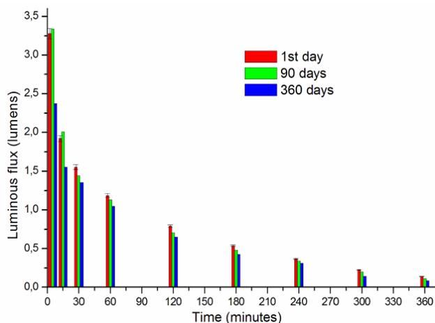
Fig. 7. The light sticks functioning - luminous flux evolution during 360 minutes since breaking.
