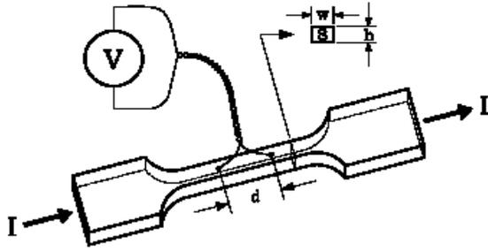
Fig. 1. Schematic representation of the sample with the electrical contacts of transport measurements  $d = 135 \mu\text{m}$ ,  $h = 400 \text{ nm}$ ,  $w = 7.53 \mu\text{m}$ .
