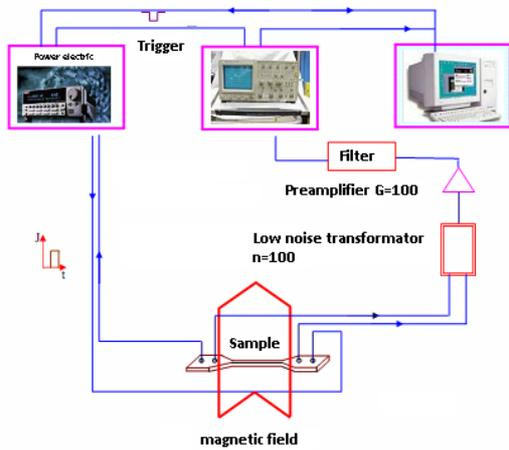
Fig. 2: Schematic diagram of transport measures to pulsed current.
