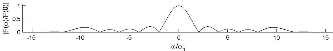
Fig. 9. The Fourier transform of  $f$  with infinite period, that is  $\Delta x \rightarrow \infty$ , not that the number of periods  $\Delta x$  is infinite.
