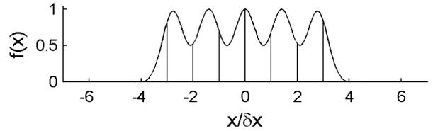
Fig. 12. Undersampled function (14 points with a minimum of 30 points).
