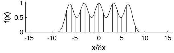
Fig. 10. Correctly sampled function (in 32 points).
