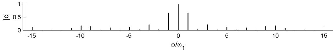
Fig. 4. The discrete amplitude spectrum of the function  $f$ , from Fig. 3 normalized to the component of maximum amplitude.
