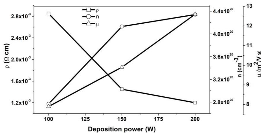
Fig. 3. The AZO films electrical resistivity ( $\rho$ ), mobility ( $\mu$ ) and carrier concentration ( $n$ ) as a function of RF power deposition
