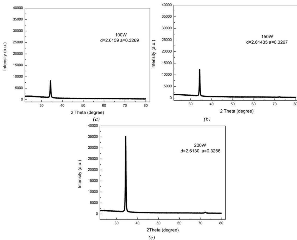
Fig. 1. The XRD pattern of AZO thin films deposited with 100 W (a), 150 W(b) and 200 W (c) RF power
