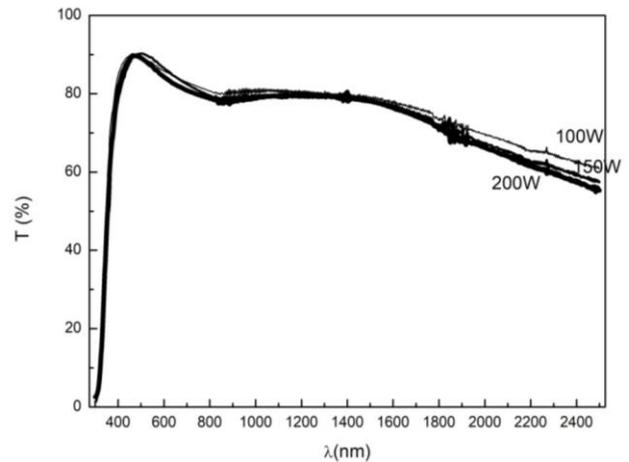
Fig. 2. The transmission variation with RF power deposition for AZO thin films
