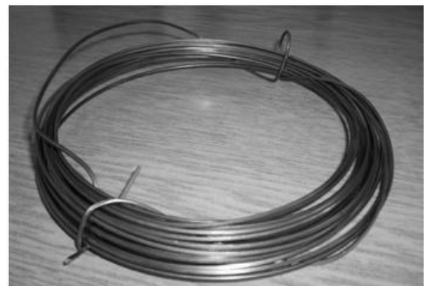
Fig. 9. View of the PdNi5-IV sample (melting and casting in the vacuum atmosphere) after rolling.
