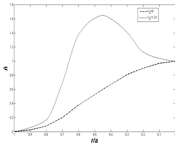
Fig. 4. The calculated profile of carriers' spatial distribution in SG MOSFET.
