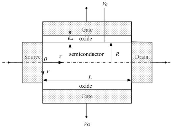
Fig. 1. Cross-sectional view of the cylindrical SG MOSFET.
