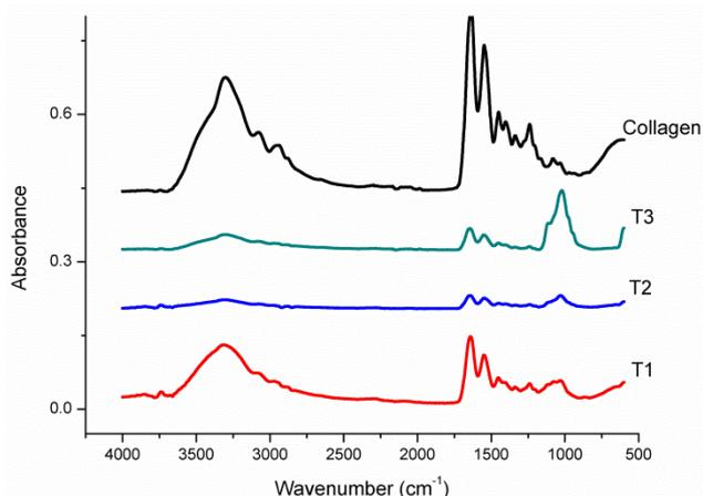
Fig. 1. FTIR spectra of the collagen:β-TCP biocomposite materials.
