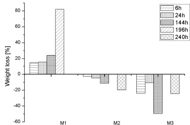
Fig. 8. Enzymatic degradation of the collagen: Mg composites.
