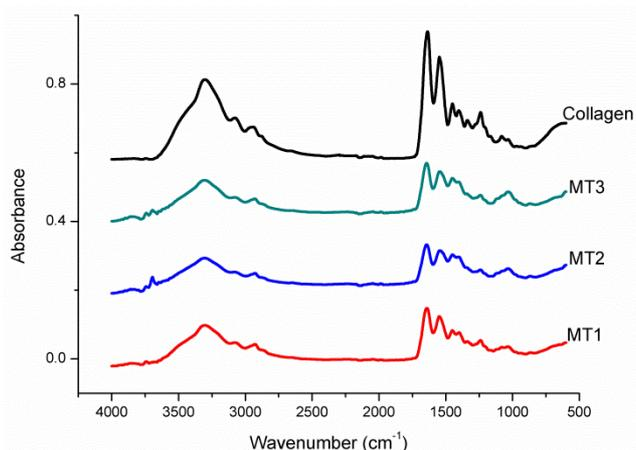
Fig. 3. FTIR spectra of the collagen:Mg +β-TCP composite materials.
