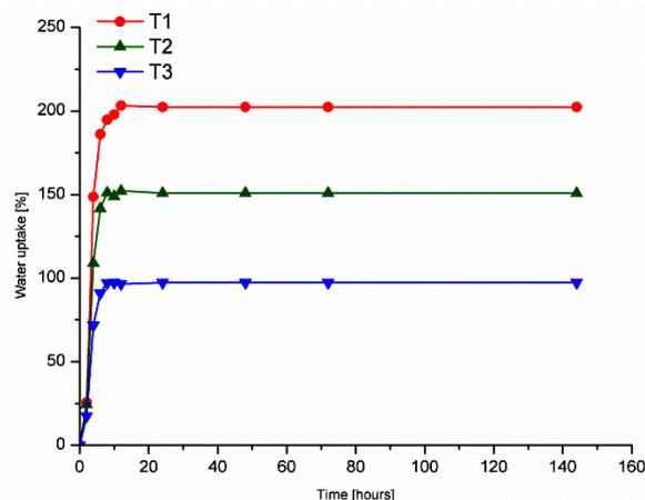
Fig. 4. Water absorption for the collagen: β-TCP composites.
