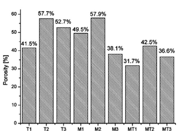
Fig. 10. The variation of the porosity with filler ratio in the experimental composite materials.
