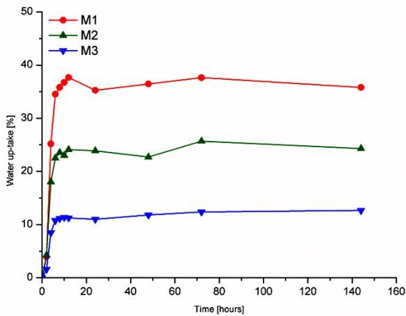
Fig. 5. Water absorption for the collagen:magnesium composites.
