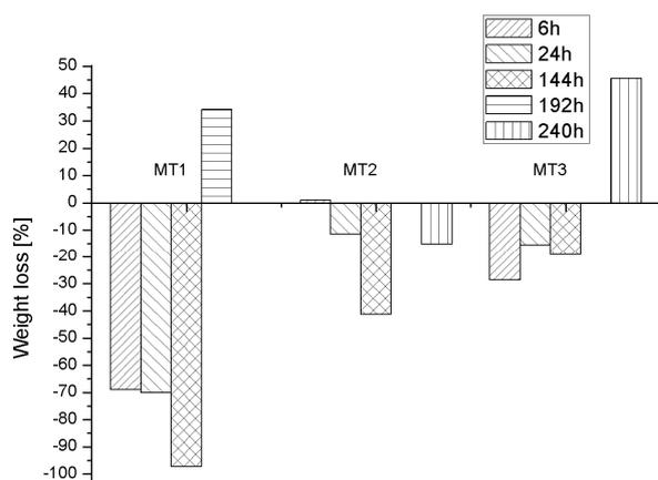
Fig. 9. Enzymatic degradation of the collagen: Mg +  $\beta$ -TCP composites.
