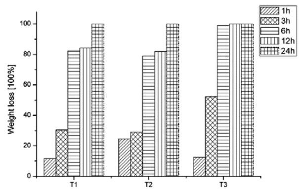
Fig. 7. Enzymatic degradation of the collagen:  $\beta$ -TCP composites.
