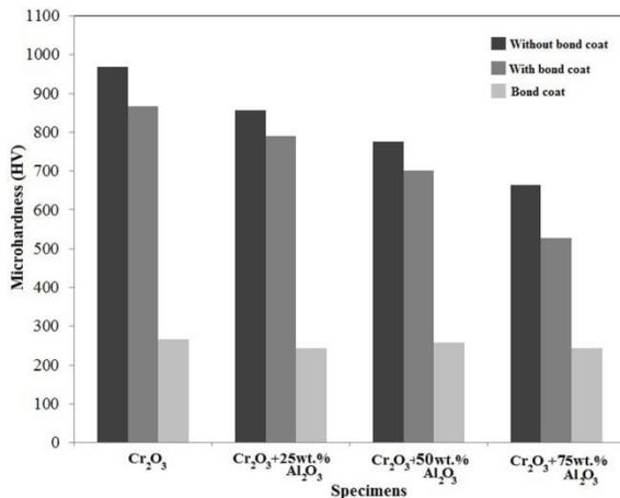
Fig. 7. Microhardness of plasma spray coatings
