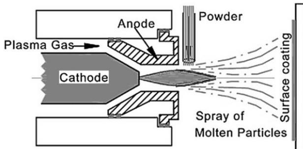
Fig. 2. Schematic cross-section of a typical plasma spray [13].
