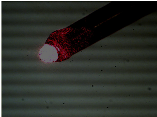
Fig. 2. The scattering of the transmitted light by spherical microlens attached to fiber. The fiber head with the lens was irradiated in the beam of an ultraviolet (UV) lamp under the condition: a) 5-7 cm distance, temperature 52 °C released by the UV beam, b) 2.5 cm distance (100 °C in the beam at the position of the microlens).
