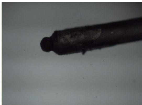
Fig. 2. The scattering of the transmitted light by spherical microlens attached to fiber. The fiber head with the lens was irradiated in the beam of an ultraviolet (UV) lamp under the condition: a) 5-7 cm distance, temperature 52 °C released by the UV beam, b) 2.5 cm distance (100 °C in the beam at the position of the microlens).
