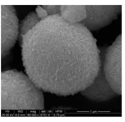
Fig. 3. SEM images of as-prepared BiOBr spherical microstructures
