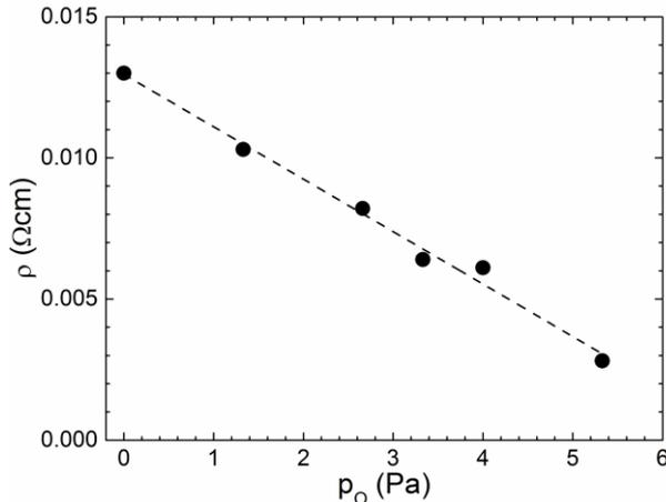
Fig. 5. Resistivity of the ZnO films as a function of the O partial pressure,  $p_O$ . The dashed line is a mathematical linear fit
