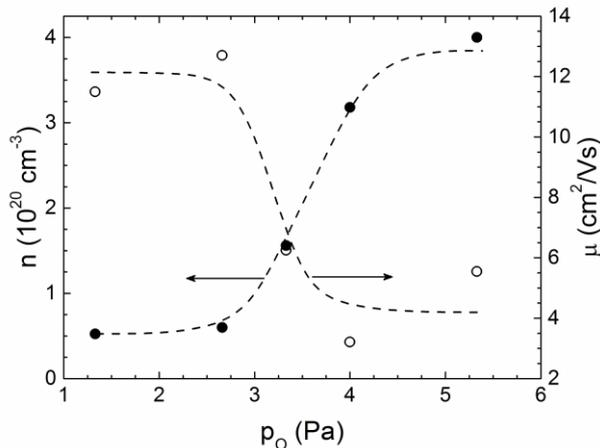
Fig. 6. Electron concentration (•) and mobility (–) as functions of the O partial pressure,  $p_O$ . The dashed curves only represent the tendency
