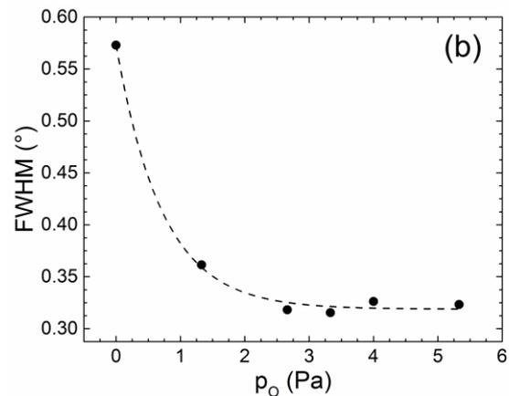
Fig. 2.  $2\theta$  angle (a) and FWHM (b) of the (002) peak as functions of the O partial pressure,  $p_{O_2}$ . Dashed lines only represent mathematical fittings
