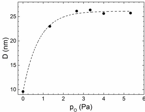
Fig. 3. Variation of the effective grain size as a function of the O partial pressure,  $p_O$ . The dashed line is an asymptotic fitting
