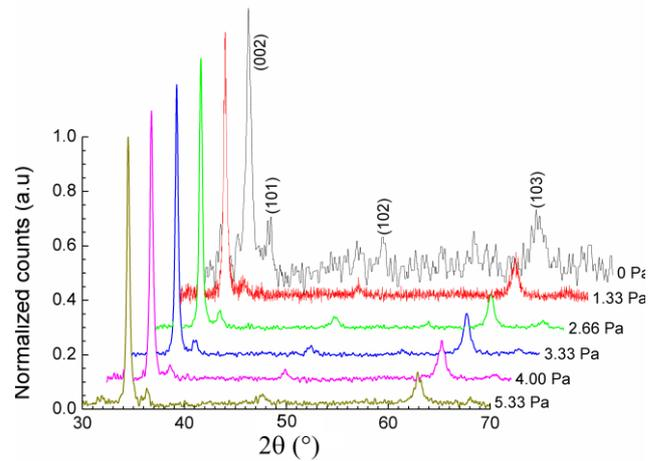
Fig. 1. Diffractograms of ZnO films as a function of the O partial pressure
