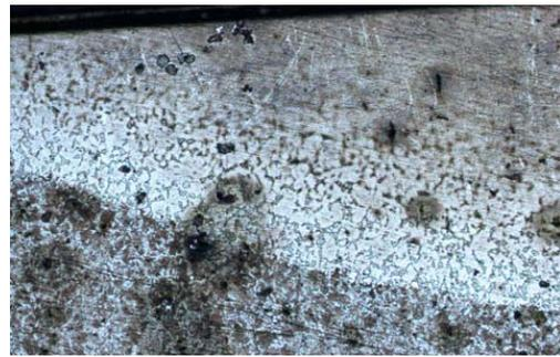
Fig.4. Steel 1.0601 improved and surface melted with CO<sub>2</sub> laser; P=800W; Nital attack; 200:1
