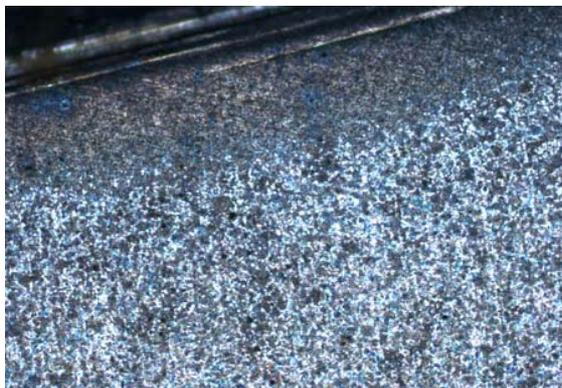
Fig.3. Steel 1.0601 improved and surface hardened with CO<sub>2</sub> laser; P=700W; Nital attack; 200:1
