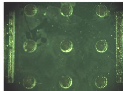
(b) Micro-thruster array for ignition
