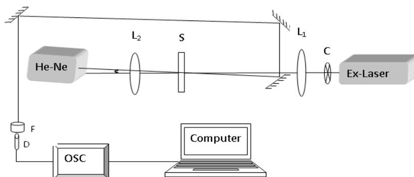
Fig.1. experimental set up of thermal lens.
