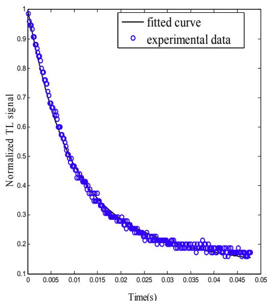
Fig. 4. Time evolution of the thermal lens (TL) signal for sample with 2% concentration. Solid line corresponds to the best fit of Eq. (1) to the TL experimental data.
