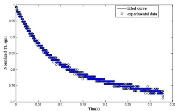
Fig. 5. The normalized TL time evolution signal for Clay. Solid line corresponds to the best fit of Eq. (1) to the TL experimental data
