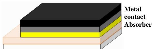
Fig.1. Schematics of a typical thin-film solar cell structure.
