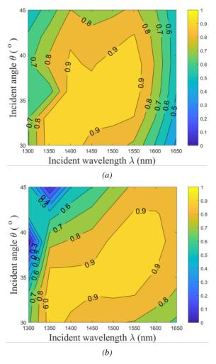
Fig. 5. Contour of the reflection efficiency of the -1st order versus incident wavelength and incident angle for (a) TE polarization and (b) TM polarization (color online)
