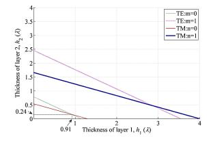
Fig. 2. The four different lines of high efficiency for both TE polarization and TM polarization on account of Eqs. (3,4) for a duty cycle of 0.7 under an operating wavelength of 1550 nm (color online)
