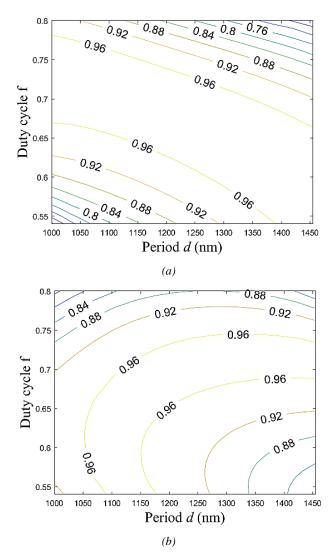
Fig. 6. Contour of the reflection efficiency of the -1st order versus grating period and duty cycle for (a) TE polarization and (b) TM polarization (color online)
