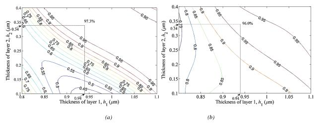
Fig. 3. Contour of the -1st reflection efficiency for (a) TE polarization and (b) TM polarization (color online)
