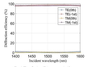
Fig. 4. The reflection efficiency versus incident wavelength for both TE polarization and TM polarization (color online)
