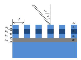
Fig. 1. Schematic of three-layer rectangular-groove metal-mirror-based grating under Bragg angle incidence (color online)
