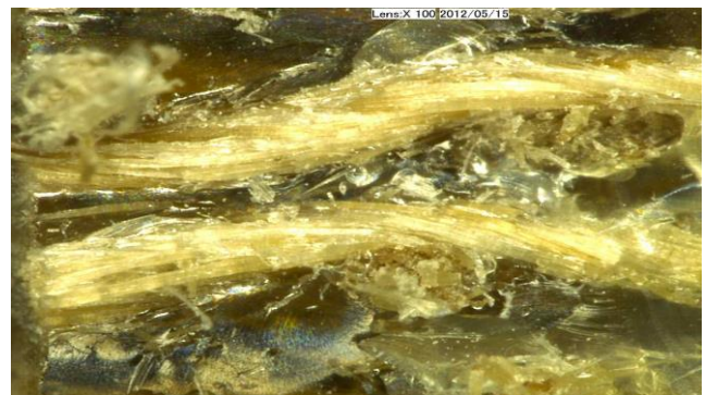
Fig. 6. Cross-section through a hemp fabric based specimen irradiated with 56.7 kGy dose (100X magnitude).
