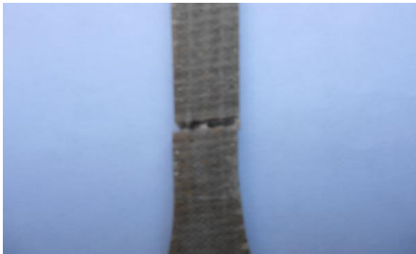
Fig. 2. Hemp fabric based specimens before and after tensile testing.
